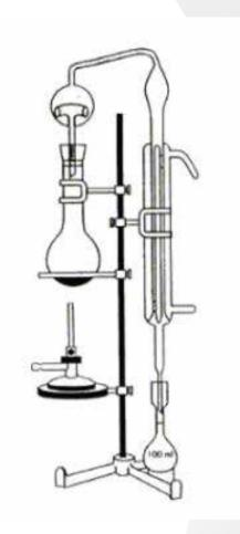
Single distiller with gas heating, according to the official EEC method. The instrument is composed of 500ml distillation flask, refrigeration unit, GS pincers, tripod with rod, support pliers, flame spreader net, bunsen with thermocouple, 200ml flask of distilled collection. Complete with 1 meter of gas pipe. The distiller can work with natural gas or LPG
