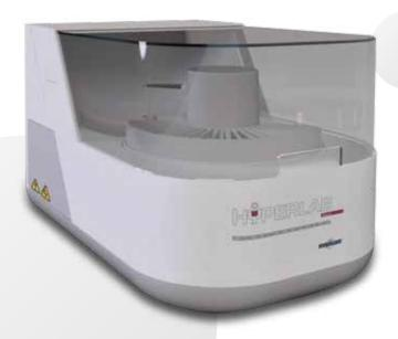
HYPERLAB SMART is a compact and versatile multiparameter analyzer designed to perform in complete automation the enzymatic and colorimetric analyses necessary to control the winemaking processes and the quality of the wine itself.
